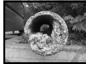
All too often fats, oil and grease are washed into the plumbing system and stick to the inside of both private and public sewer pipes. Over time the oil and grease build up and eventually blocks the entire pipe causing sewer backup and overflow.
